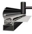
Tap the EZY-Grip™ with a light rubber mallet, locking the fabric into the V-Grip channel.
